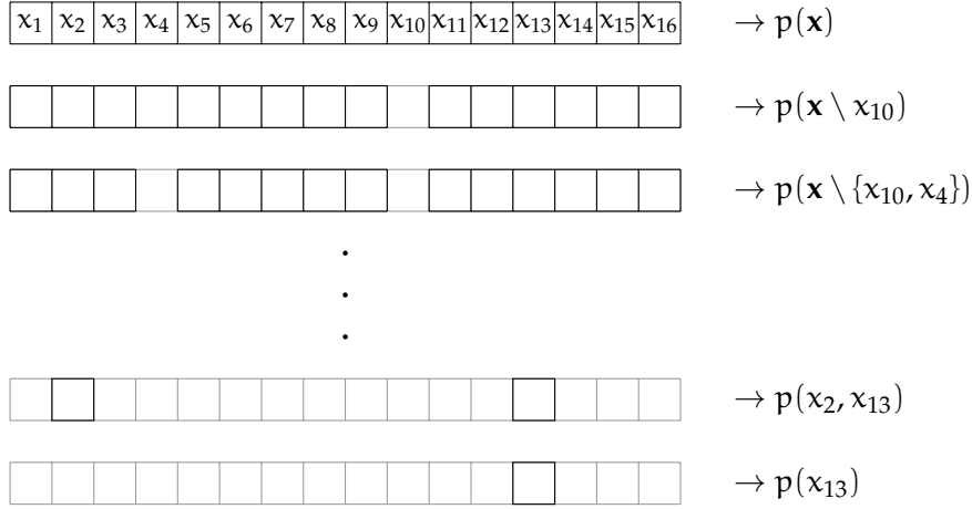
FIGURE 4.5 – In a feature clipping process, one of the features \{x_1, x_2, \dots\} is sequentially removed from the training and prediction stage of the regressor. The rule, which decides what feature is removed in the next step, is called the clipping order.
